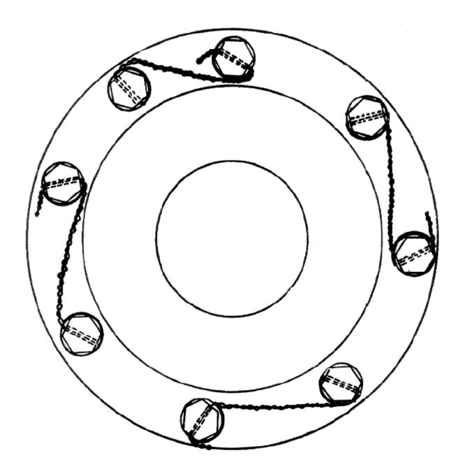
Double lace as shown, using soft stainless steel lacing wire approximately .041" in diameter.
