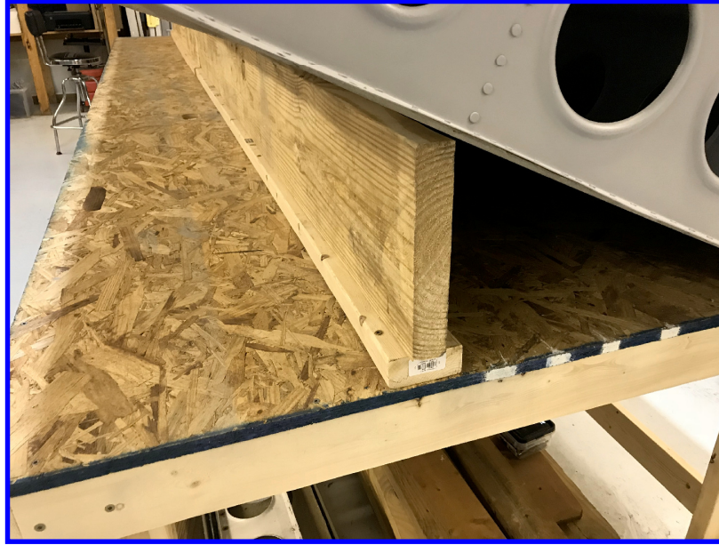
End view of wing support for aft spar installation. (2 ea. 2 x 8 and 2 ea. 2 x 4)
