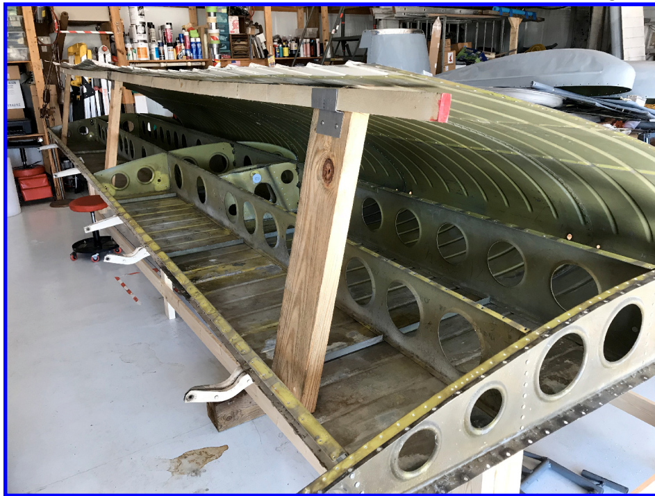
Wing opened up on the wing table. This allows full access to everything.
