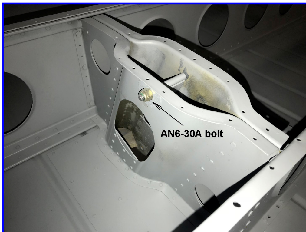
Wing Float Socket with bolt and the "key" below the bolt.
