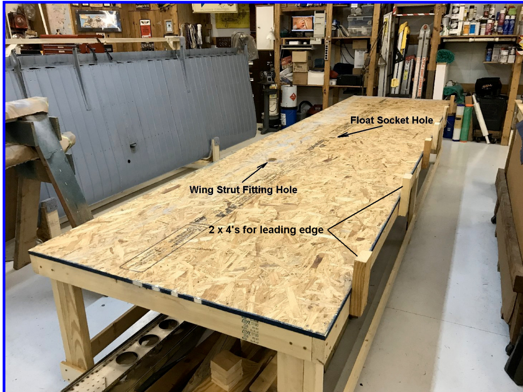
Wing table – Notice 2 x 4's for holding the leading edge in place and holes for fittings.
