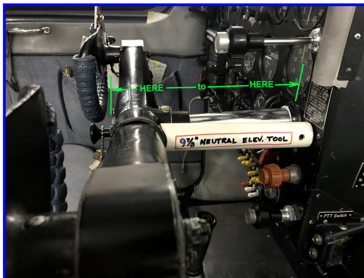
PVC Neutral Elevator Tool; cut to length that keeps elevator neutral
