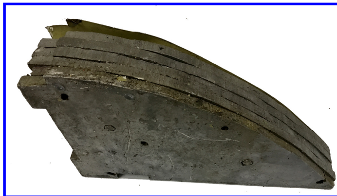
Republic-installed lead weights at Sta. 4.5
