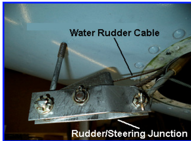
Rudder/Steering Junction (Shown for clarity only. No need to remove it from the Seabee)
