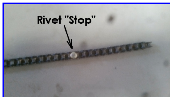
Photo of rivet "stops" on forward chain. Same chain; two rivets. (Photos by member Jaren Lynn)
