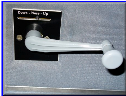
Trim Handle with trim indicator. Indicator shows slight nose up trim.
