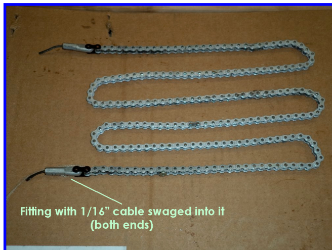
Forward Chain with rivet "stops"
