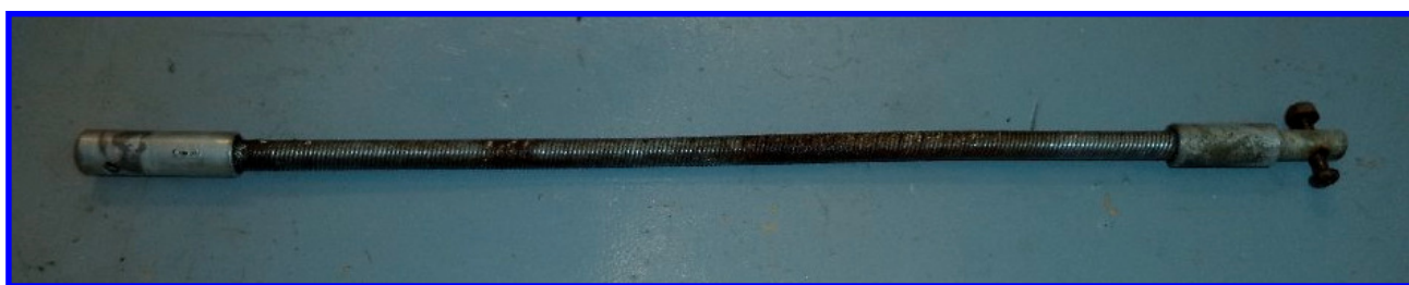
Flexible cable attached to each trim gearbox from the rear sprocket
