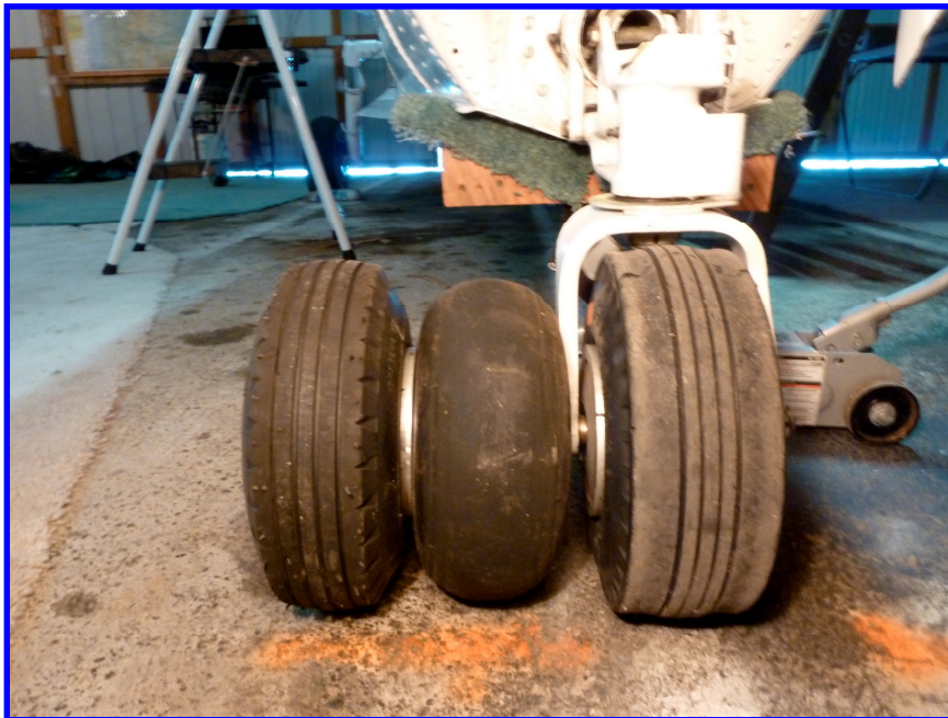
Three of the 4" tires available (Left to right: StoA 10 x 350 x 4 (4") (Desser Tire Co.) 10.00 SC (3" smooth contour) 10.5 x 4 (4") (channel tread) the old and famous
