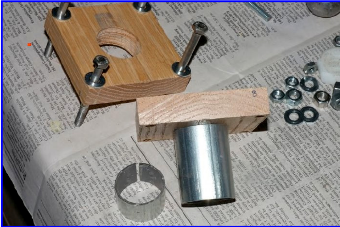
Forming tool parts. Large tube must fit tight.
