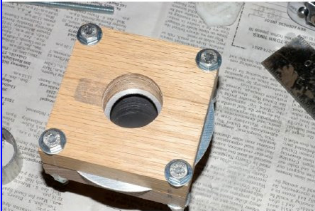
Disc in place ready for clamping in forming tool (top photo) Slit spacer removed ready for 1-5/16" ball AFTER the spacer is removed (bottom photo)
