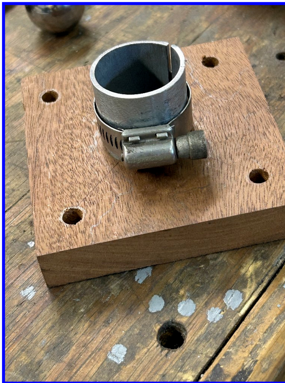
Hose clamp used for closing the gap on small tube. Remove when in place. (flush with the blank spacer)
