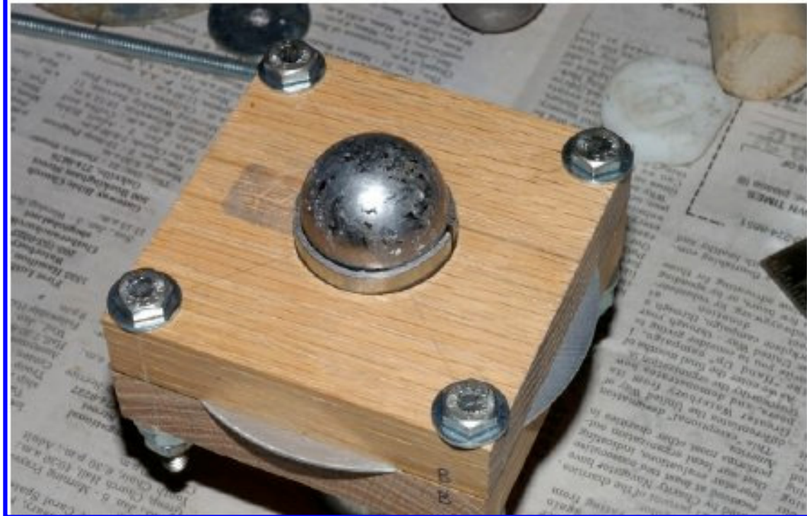
Disc clamped in forming tool (top photo) 1-1/4" ball in place ready for first forming step (bottom photo)
