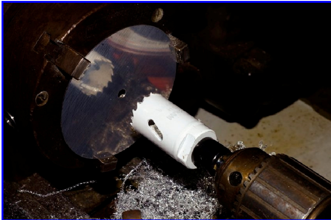
Drilling large center hole (1-1/8") on a lathe
