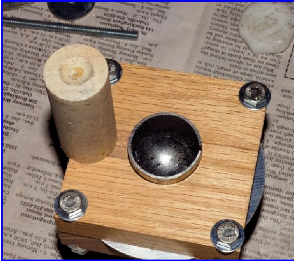
Forming tool with dowel pusher. Note depression in the dowel. 1-1/4" ball is shown.
