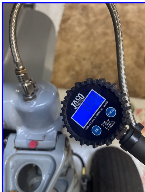
Fill the strut with Nitrogen
