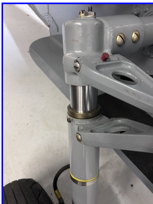
Strut fully collapsed
