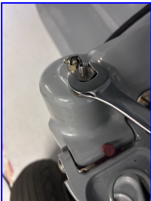
3/4" open end wrench, remove Schrader valve housing
