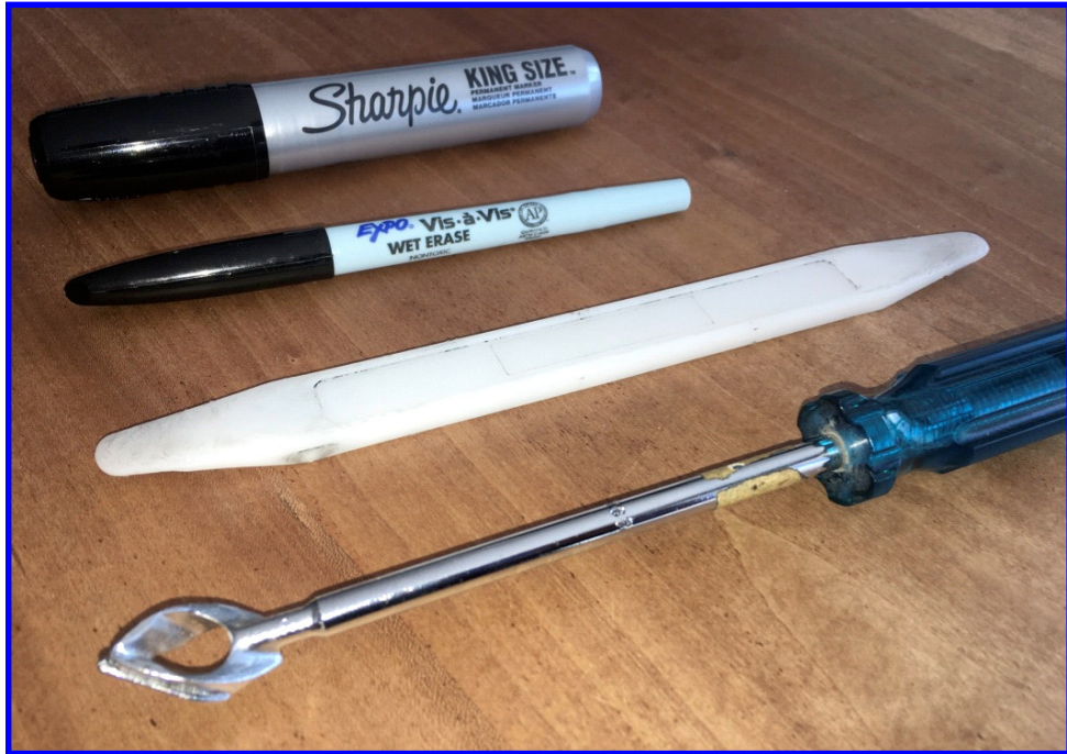
From top to bottom: King Size Sharpie; wet erase marker; window install tool; rare locking strip installation tool. Note profile of head for both seal track and lock strip.
