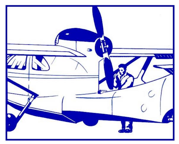
Check the fluid level in the brakes, oleos and hydraulic systems and replenish where necessary.
