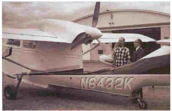
George Pappas (left) produced the first Lycoming conversion including a new metal cowl. Pappas made many other refinements to his Seabee.
