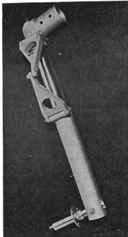
Seabee main landing gear strut. New production version of this unit has simple elbow fitting for attachment to hull shaft.
