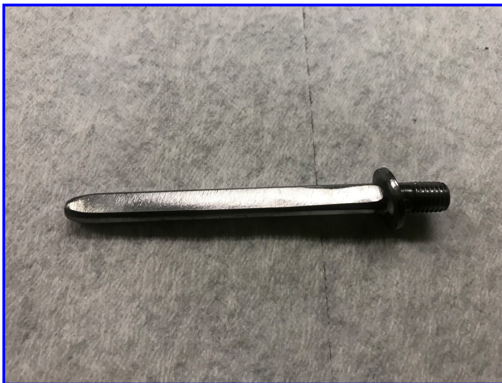
Completed pin with "flat". Note rounded end of pin.
