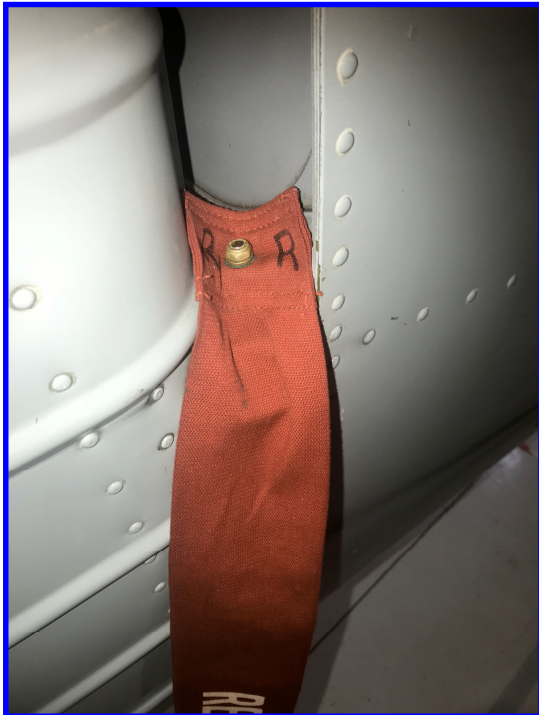
Air rudder lock installed
