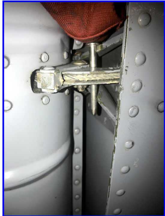
Note where pin locks between horn and airframe.
