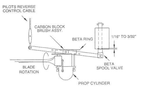
The most common indication of incorrect rigging of the beta spool valve is the inability of the propeller blades to come out of high pitch at start up. Excessive manifold pressure will be required to achieve run-up RPM and the prop pitch control will be ineffective.
