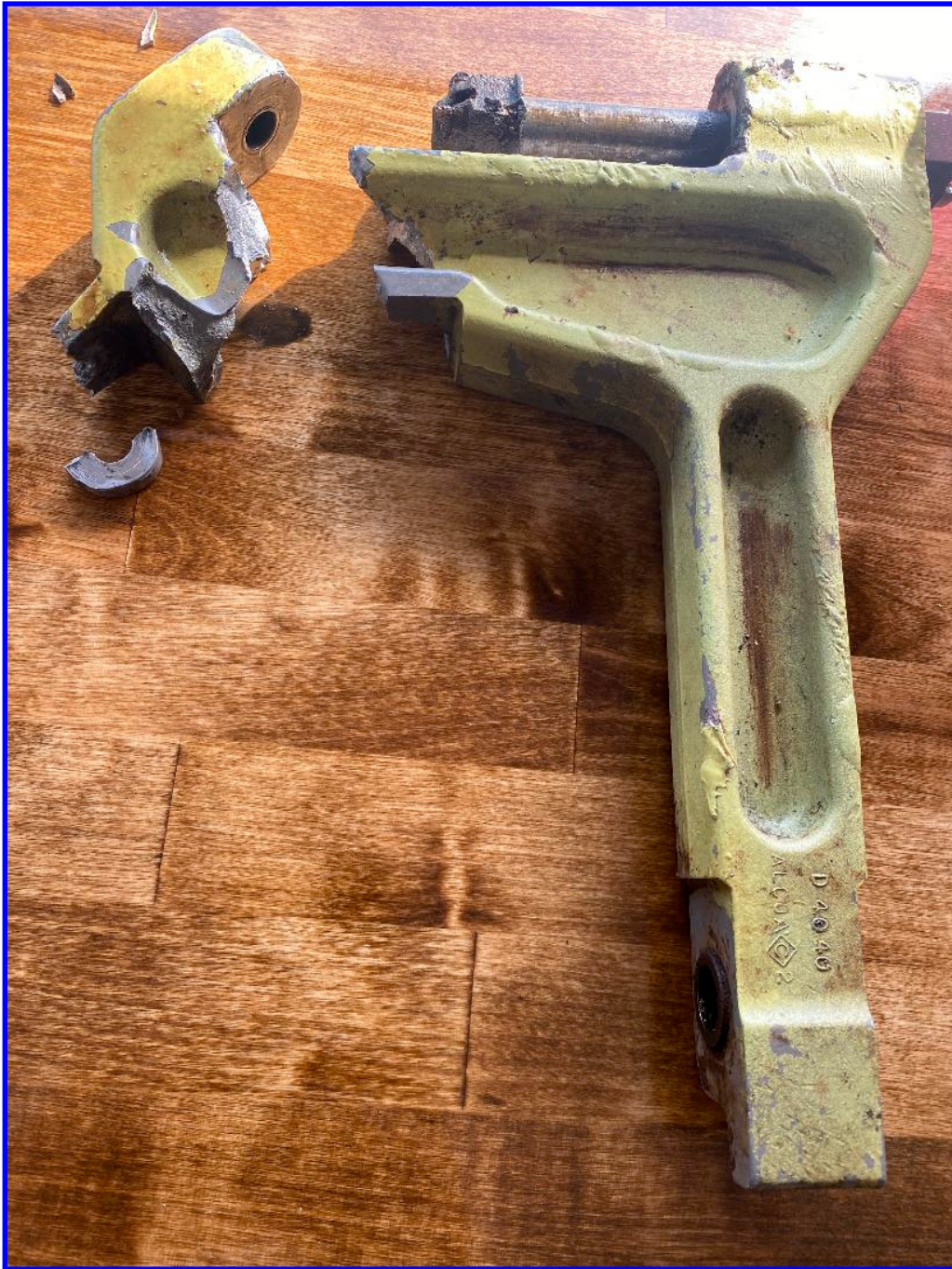
Broken "H" bracket (Part 1112)
