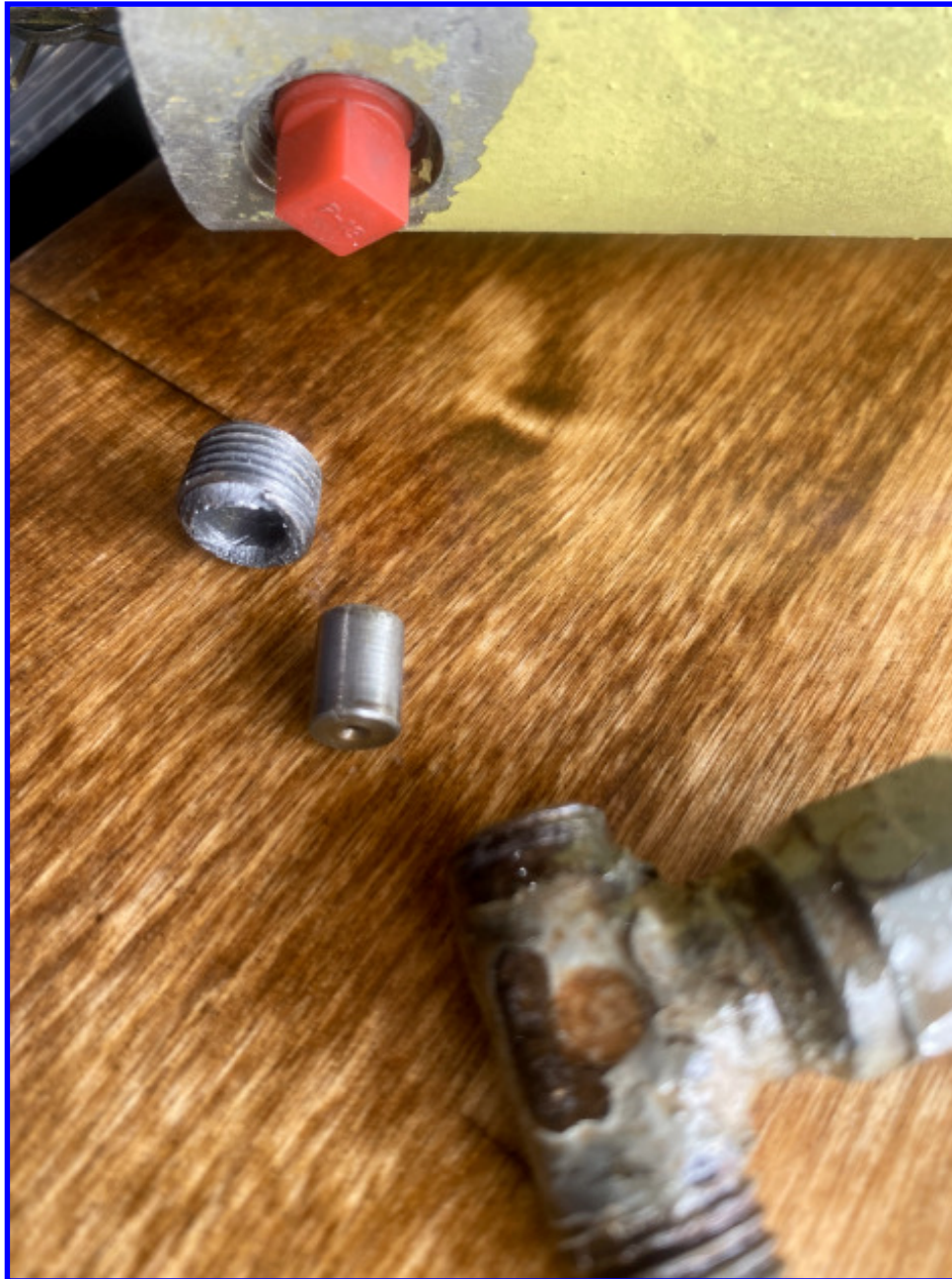
Broken fittings on landing gear actuator
