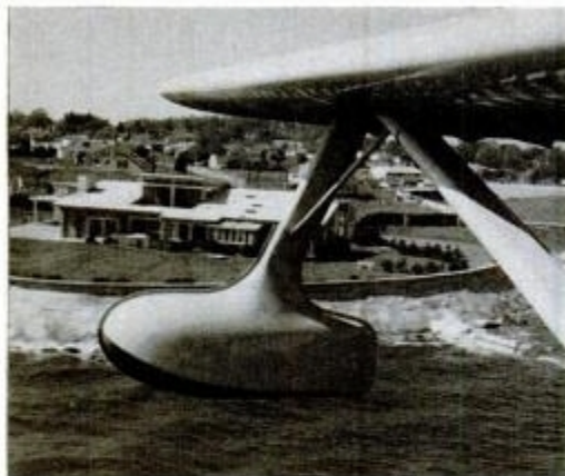
The pontoons, made from two half-sections fastened together, are typical of the Seabee's simplified construction. The instrument panel spans only half the cockpit, permitting use of the passageway to the bow door. The right control wheel is easily removable.
