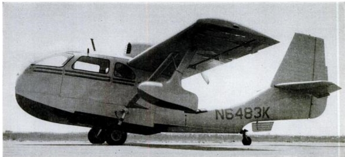
Proud and sturdy, provided there's no hidden corrosion. The tailwheel is steerable, full swiveling beyond a certain limit. Cabin has three doors.
