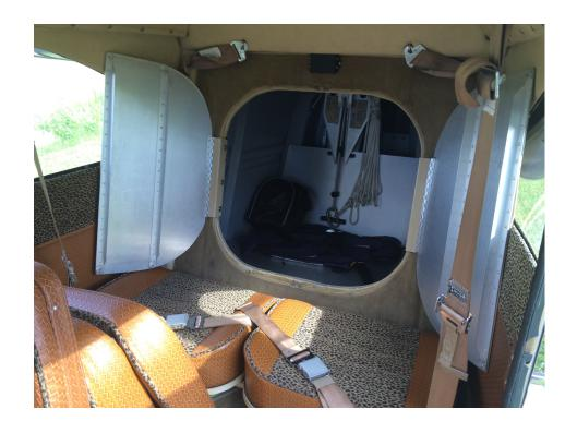
Enlarged cargo doors for loading and access to electrical bay & anchor.
