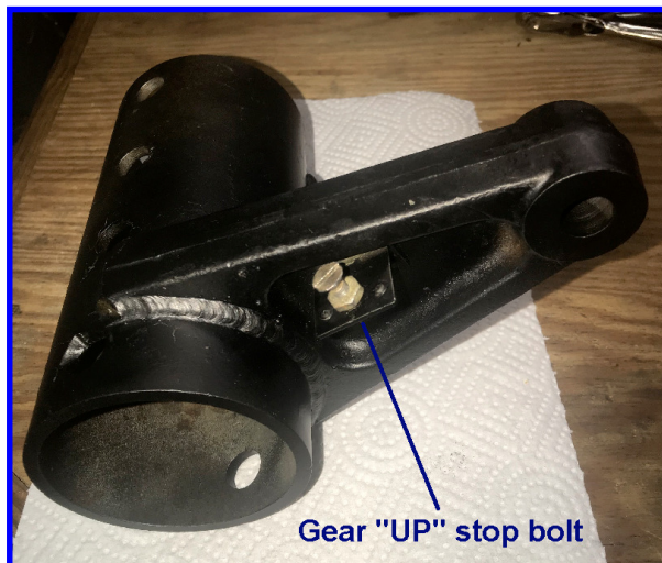
Coupling with gear "UP" stop bolt shown (This is my spare)
