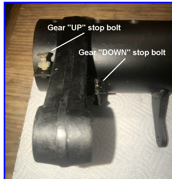
Coupling showing both "UP" and "DOWN" stop bolts
