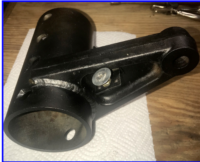
Center coupling with modified stop bolt
