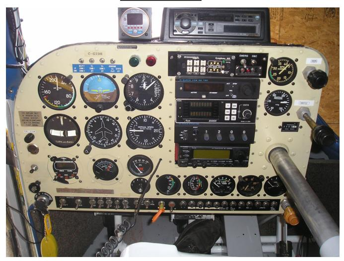
AVIONICS: NARCO Com 810 VHF, NARCO AT50 Transponder, ICOM IC-2000 programmable FM, DRE Communications Symphony 468 Audio Panel Apollo 604 Ioran. Latitude Sentinel Satellite tracking system. Flowscan 450 Fuel Flowmeter, Pelco Closed Circuit Twin Camera System (one wing mounted, one cockpit mounted), Six position EGT Pelco MPT9500 Camera Controller & LCD Screen, Alpine Recorder / stereo player, 6 CD changer & Four Place headsets (Lightspeed noise attenuating).
