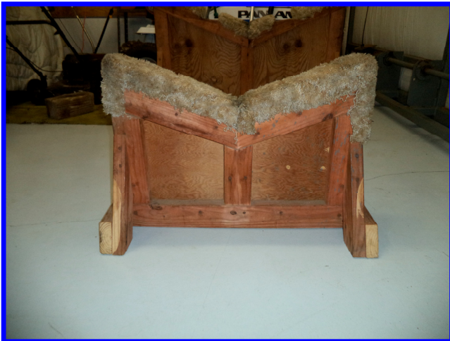
Forward Hull Stand ↑ Aft Hull Stand ↓ (note plywood "sandwich")
