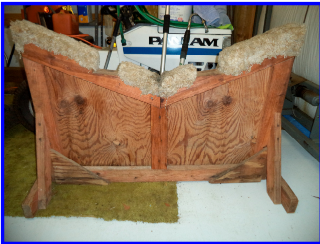
Forward Hull Stand ↑ Aft Hull Stand ↓ (note plywood "sandwich")
