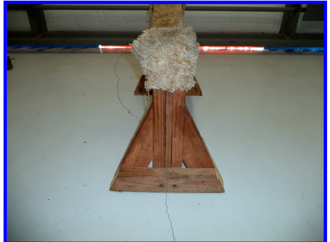
Forward Hull Stand ↑ Aft Hull Stand ↓ (note plywood "sandwich")
