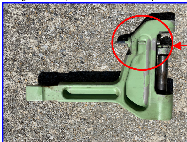
H-Bracket as removed from landing gear mechanism
