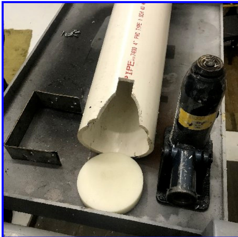
Lower components of Franklin Prop Jack (L to R: Jack retainer, 4" PVC pipe with piston, bottle jack)
