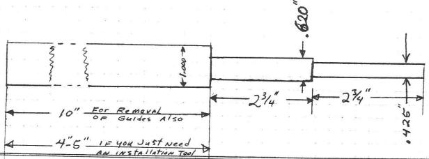
AFter Cyls Cool- Finish Ream Guide on Drill press, Turning Reamer dead Slow, or by hand, to Finish Size of . 4365". This will give about .003" clearance between Value Stem & Guide.
