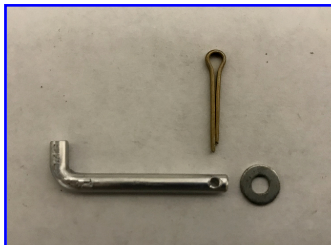
Cable guard pins with washer and cotter pin
