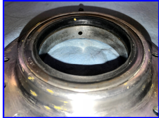
Bearing shown with grease hole. Seal is above the bearing
