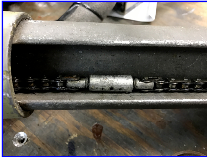
Control Arm cover removed showing turnbuckle and chain. Safety wire removed.
