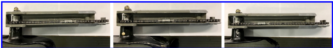
Turnbuckles in correct position Aileron Centered
