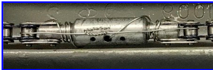
Turnbuckle and chain safety wire installed. THIS IS REQUIRED!
