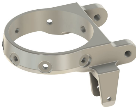
CAD rendering of proposed collar (RPN 1126 or 17F42041)
