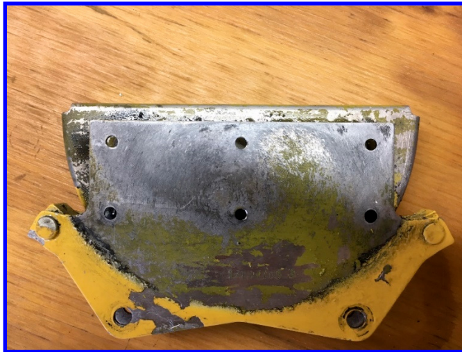
This is the horn with one nose rib removed. It is sandwiched between two.
