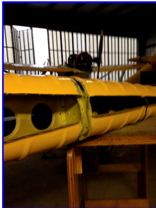
These are the leading edge rivets removed
