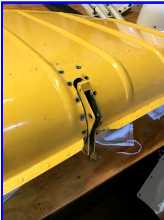
These are the nose-rib-to-skin rivets removed
