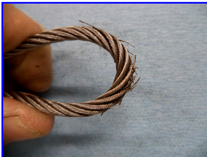
Cables appeared good until they were bent!
