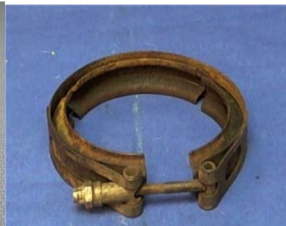
3 segment, coupling removed from service
