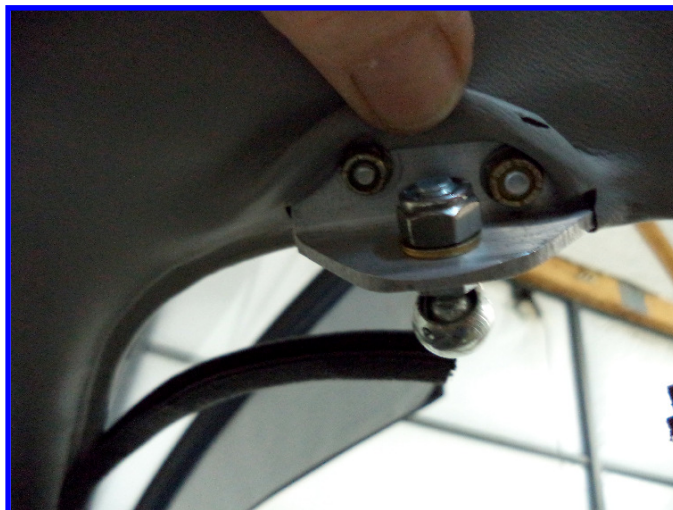
Lower Bow Door Fitting, ball end installed
