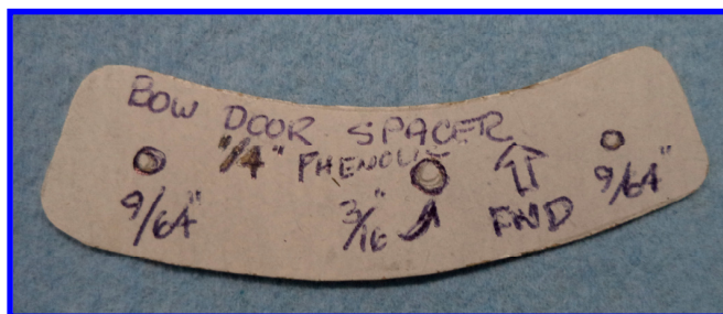
Phenolic Upper Fitting Spacer (Actual size)
