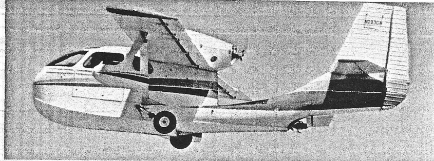
Above: Demonstrating the geometry of its undercarriage is N283GM and, below, Canadian "Thunder Bee" C-FOME fitted with a 320hp Chevrolet Corvette engine.
