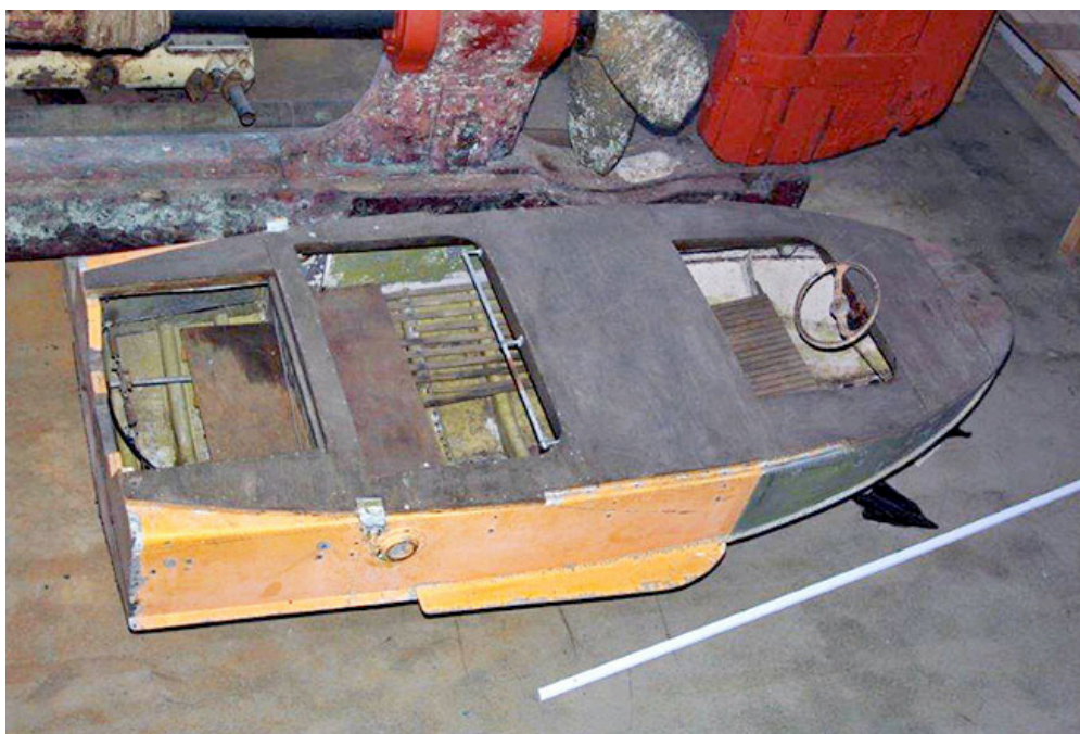
The hull of VT-CST, still with Seabee water vane on each side, rebuilt as a home-made boat. Photo by Dave Eyre
