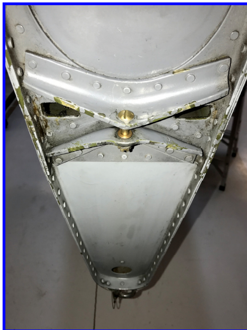
Lower Rudder Control Horn Pivot (Note Oilite bushings)
