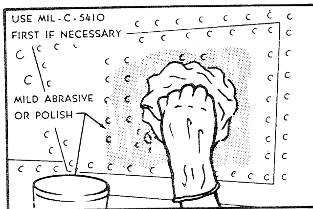
FIGURE 6-12. POLISHING AND BRIGHTENING ALCAD SURFACES
