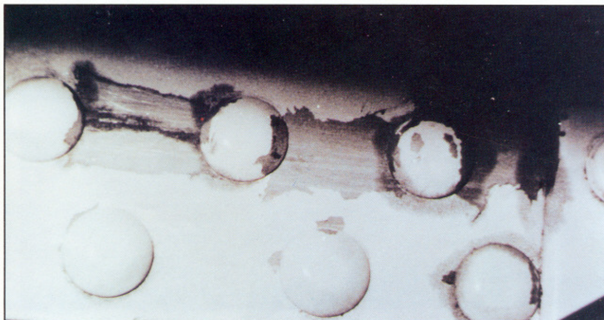
FIGURE 5-6. CORROSION CRACKING BETWEEN FASTENERS ON A WING SPAR
