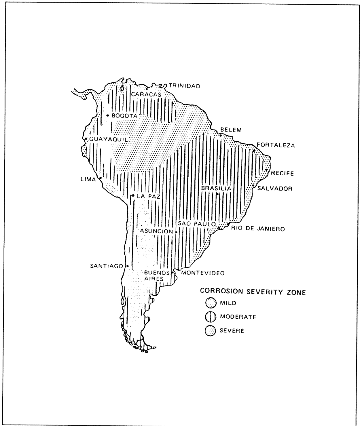
FIGURE 4-16. SOUTH AMERICA CORROSION SEVERITY MAP
