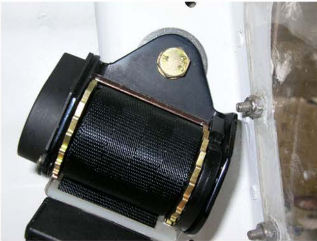
Rear shoulder harness reel mounted (typ)
