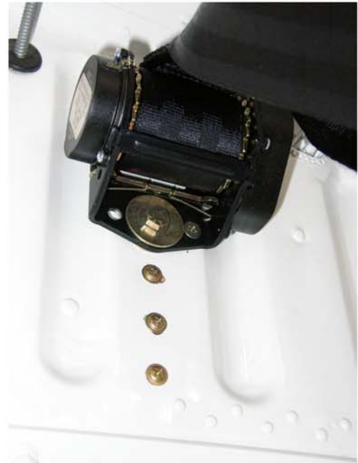
Front shoulder harness reel mounted (typ)
