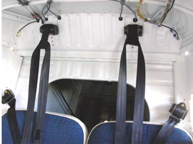
All shoulder harnesses in place
