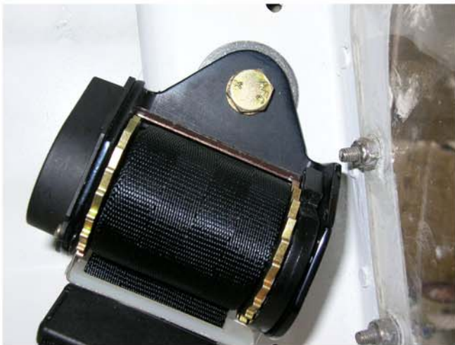
Rear shoulder harness reel mounted (typ)
