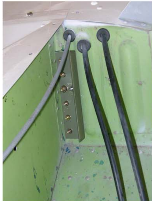
Front shoulder harness reel doubler - right side.
