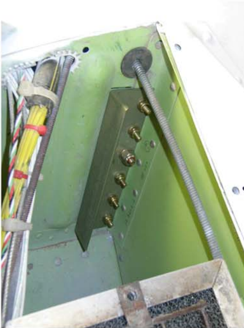
Front shoulder harness reel doubler - left side.
