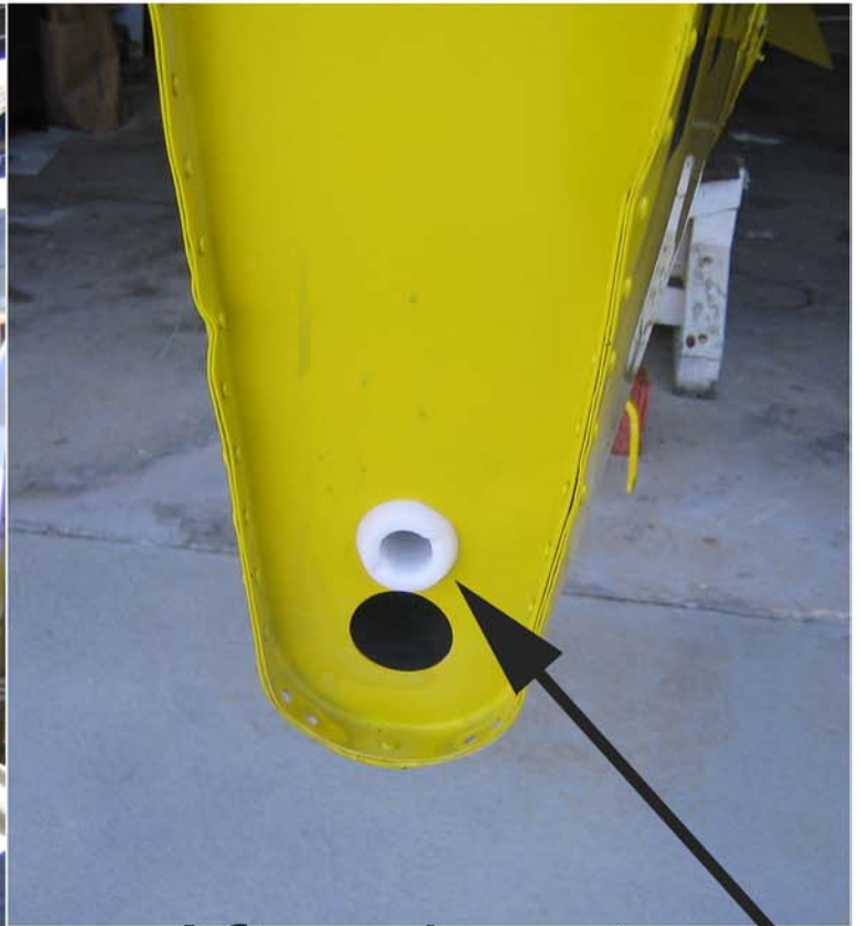
Aft and center bilge pump outlet
