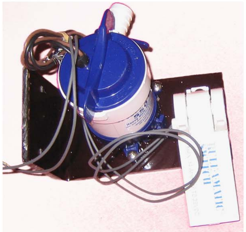
Bilge pump and switch on mount (typical)
