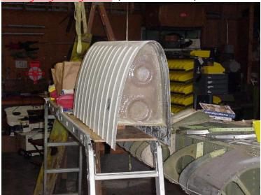
Second generation Seabee Guru, Henry Ruzakowski, has developed tanks that will hold at least 15 useable gallons per side. They are made of carbon fiber and Kevlar and will gravity feed to the main tank with the operation of one lever. They will be done on a field approval, so you'll have to take your airplane to him in Florida. So, let's plan a trip to Sun and Fun!!! Call or email Henry for more information. 561-436-0821 amphibs1@aol.com
