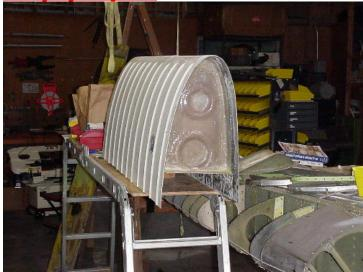
Second generation Seabee Guru, Henry Ruzakowski, has developed tanks that will hold at least 15 useable gallons per side. They are made of carbon fiber and Kevlar and will gravity feed to the main tank with the operation of one lever. They will be done on a field approval, so you'll have to take your airplane to him in Florida. So, let's plan a trip to Sun and Fun!! Call or email Henry for more information. 561-436-0821 <a href="mainto:amphibs1@aol.com">amphibs1@aol.com</a>
