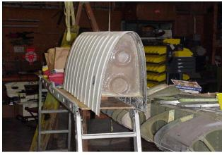
Second generation Seabee Guru, Henry Ruzakowski, has developed tanks that will hold a least 15 useable gallons per side. They are made of carbon fiber and kevelar and will gravity feed to the main tank with the operation of one lever. They will be done on a field approval, so you'll have to take your airplane to him in Florida. So, let's plan a trip to Sun and Fun!!! Call or email Henry for more information. 561-436-0821 amphibs1@aol.com
