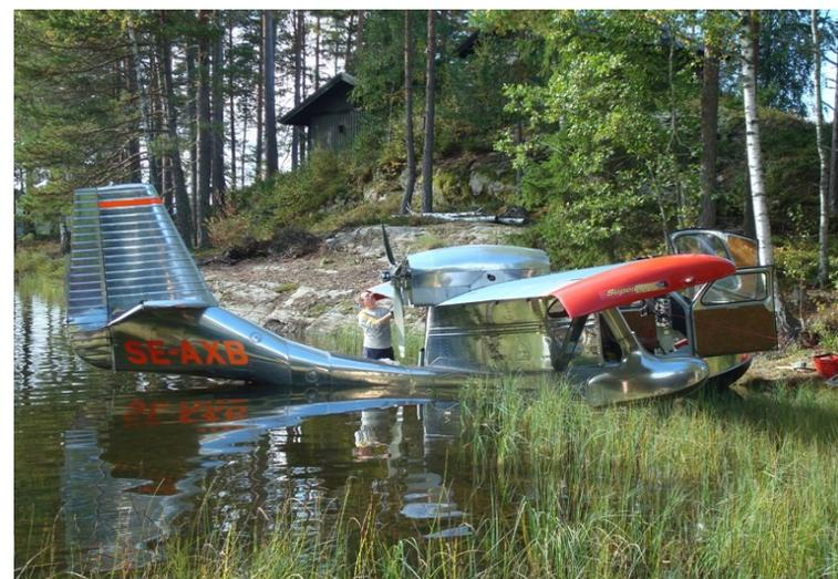
away early in the 1950's. Means that I have a very light Seabee ( empty weight 2000 lbs ) / Simuflight conv. / long wings / extended flaps. Yes I have Com. GPS. Mode C Transp. and 26.5 v Gyros.
