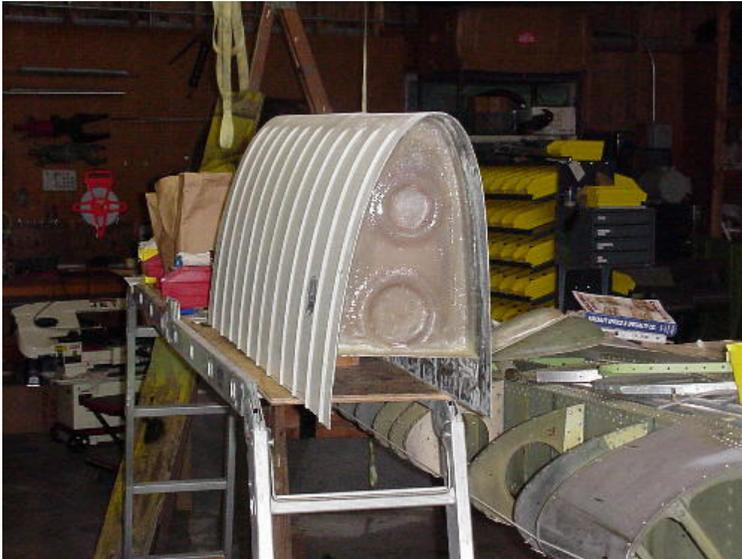
Second generation Seabee Guru, Henry Ruzakowski, has developed tanks that will hold at least 15 useable gallons per side. They are made of carbon fiber and Kevlar and will gravity feed to the main tank with the operation of one lever. They will be done on a field approval, so you'll have to take your airplane to him in Florida. **So, let's plan a trip to Sun and Fun!!!** Call or email Henry for more information. 561-436-0821 [amphibs1@aol.com](mailto:amphibs1@aol.com)
