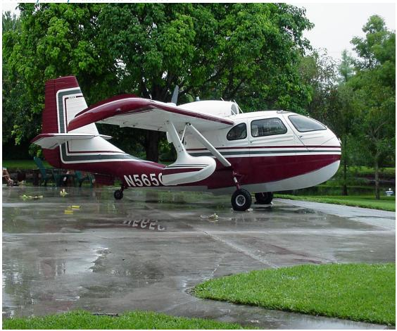
RC-3 SEABEE '47 1370TT LYCOMING GO-480 630 HRS SMOH. PROP 540 SMOH. (5 YR INSP AD97-18-02-R1 COMPLETED 6/27/06) STOL conversion w/fences & droop tips. 2 batteries w/series start. extended spray rails, ldg lts, Cleveland brakes, electric hydraulic pump for gear & flaps, shoulder harnesses front seats, ovrhd engine controls, Terra TRT250 Transponder, ?AT3000 Altitude Encoder, Garmin 250XL GPS with Comm, Appollo Iso Amp and Comm. \$110K ?NY (ELM) 607-739-3275 or 570-297-5076.? clyder@epix.net 1
