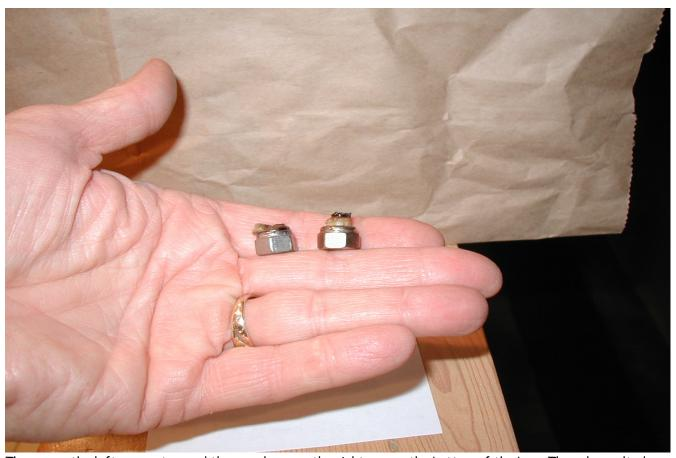
The one on the left was on top, and the one shown on the right was on the bottom of the bus. The nylon melted, causing the connection to become loose. Pretty simple, but I can't tell you the countless hours I've screwed around with this. I don't care if Nylocs are approved, I don't feel they should be used in the engine compartment or on electrical stuff.
