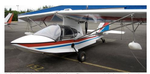
Options include; Hydraulic gear, Heel brakes, Electric trim, Whelen strobes, King com radio, King transponder, 121.5 mHz ELT, Nav lights. Rotax 914.turbocharged engine 115 hp. Full electrical system. Dual electric fuel boost pumps. 137 total hours. Built by an A and P mechanic. Always hangared. \$45,000. (A new Rotax 914 sells for \$31,000 by itself.) Contact Tom Watkins 253-549-4549 Cell 602-284-0770. 8/09
