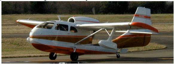
Recent engine overhaul. New 3 bladed Hartzel propeller with Beta Ring pitch control, fully reversible. Droop tip extended wings. Collins microline VHF, transponder, ADF. VIR and Morrow Apollo Loran C. Digital fuel management system Miniflo L. Steerable tail wheel. To inspect airplane, call (253)752-4987 to arrange an appointment. Ben Blackett <a href="mailto:wbnsurgconsult@comcast.net">wbnsurgconsult@comcast.net</a> 02/10
