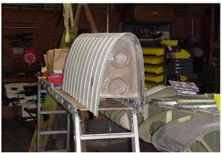
Second generation Seabee Guru, Henry Ruzakowski, has developed some <u>leading edge wing</u> <u>tanks</u> that will hold a least 15 useable gallons per side. They are made of carbon fiber and kevelar and will gravity feed to the main tank with the operation of one lever. They will be done on a field approval, so you'll have to take your airplane to him in Florida. So, let's plan a trip to Sun and Fun!!! Call or email Henry for more information. 561-436-0821 <u>amphibs1@aol.com</u>
