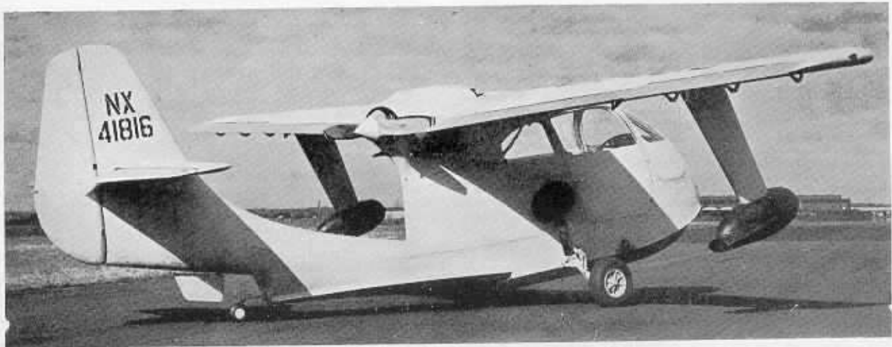
The Republic Seabee Light Amphibian Flying-boat (175 h.p. Franklin engine).
