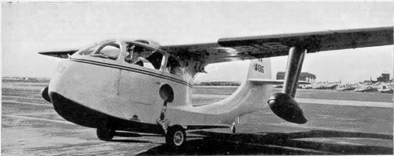
The Republic Seabee Light Amphibian Flying-boat (175 h.p. Franklin engine).
