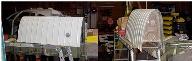
Second generation Seabee Guru, Henry Ruzakowski, has developed some <u>leading edge wing tanks</u> that will hold a least 15 useable gallons per side. They are made of carbon fiber and kevelar and will gravity feed to the main tank with the operation of one lever.
