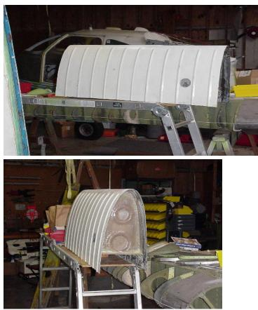
Second generation Seabee Guru, Henry Ruzakowski, has developed tanks that will hold a least 15 useable gallons per side. They are made of carbon fiber and kevelar and will gravity feed to the main tank with the operation of one lever. They will be done on a field approval, so you'll have to take your airplane to him in Florida. So, let's plan a trip to Sun and Fun!!! Call or email Henry for more information. 561-436-0821 <a href="mailto:amphibs1@aol.com">amphibs1@aol.com</a>
